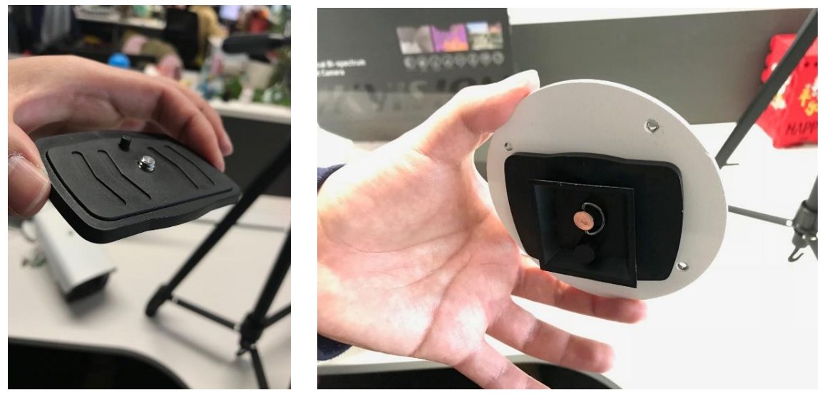
A. Tripod connector fixed on the adapter
