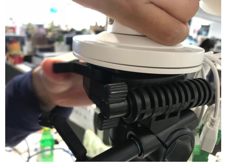
C. Install the camera on the tripod
